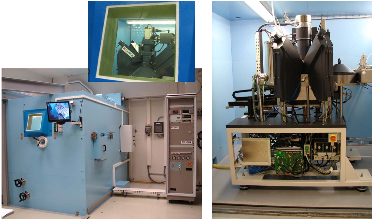
Views of the Cameca SX100R electron microprobe analyser for the analysis of highly irradiated materials at the Institute for Transuranium Elements.
