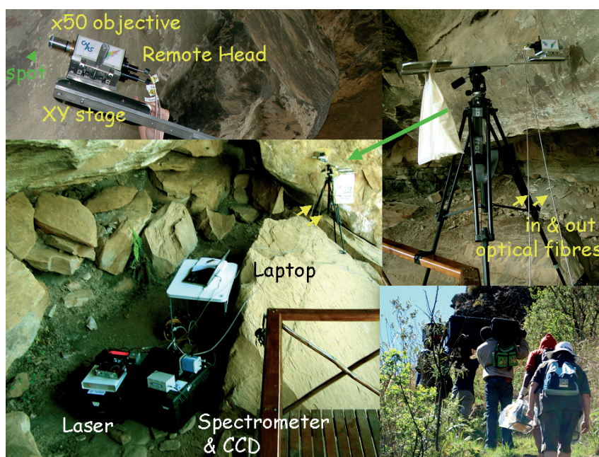
Figure 3. Examples of the versatility of Raman microspectrometry: a) use of mobile Raman spectrometer and laser source to study rock art in Draggensberg National Park (South Africa; Photograph A. Tournié) [15]; b) the laser beam is focussed on a single silk fibre under controlled axial tension and soaked in water (Photograph P. Colombari) [13, 16].
