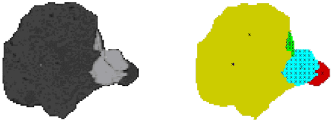
Figure 10. Particle with quartz (dark grey) and sulphides (light grey). An X-ray map is performed on the sulphides only to distinguish chalcopyrite (blue) from pentlandite (green).
