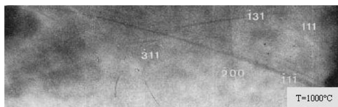
Figure 8. Measured Fe lattice constants versus temperature ( \alpha - \gamma transformation) as well as Kossel pattern of \gamma -iron at 1000°C: two grains [26].
