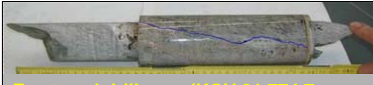
Fractured drill core (KOV 01 774.7-775.2) (core #8)
