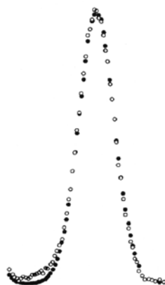
Fig. 23. Plot of an experimentally acquired X-ray peak (open circles) and a fitted Gaussian curve (closed circles), showing the low energy tail in the experimental curve which results from incomplete charge collection.
